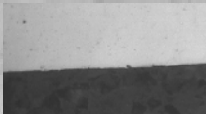
Glass-filled epoxy for edge retention
